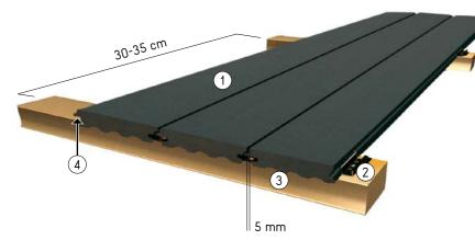
patent IP1.452.665 (3) Hard wood or aluminium joists
